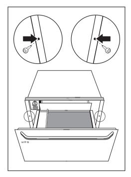
Open the plate warmer drawer and use two screws to secure the plate warmer to the side walls of the cabinetry.
